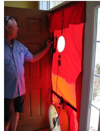
Figure 5. Blower door test.
